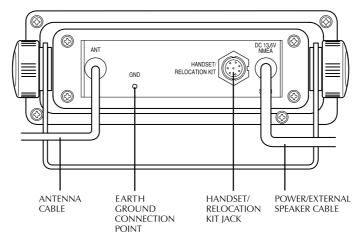
Figure 3-1 Rear Connections
